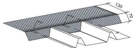
Can be Utilized on Flat Metal Roofing Profiles (e.g Patios, awnings, pergolas etc.) Flat piece of 200mm Wide with a 70mm downturn. Designed for you to custom cut to suit your needs.
