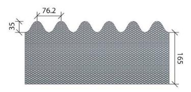
The Signature Product of Corrugated Gutter Guard. Standard Width of 200mm. Caters for all corrugated roof and gutter combinations. Also Available in reverse format for high pitch situations of for more efficient capture of rainwater.
