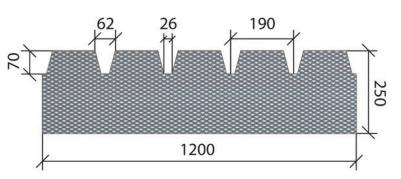
Signature product, pre-cut, folded and designed to suit: Lysaght Trimdek<sup>®</sup>, Stramit Monoclad<sup>®</sup>, Metroll Trimclad<sup>®</sup>, Stratco Superdek<sup>®</sup>.
