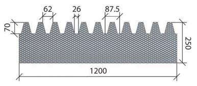
Product is precut and designed to suit: Varying roof profiles. Suits Metroll MetroSpan<sup>®</sup> and Stratco Smartspan<sup>®</sup>.
